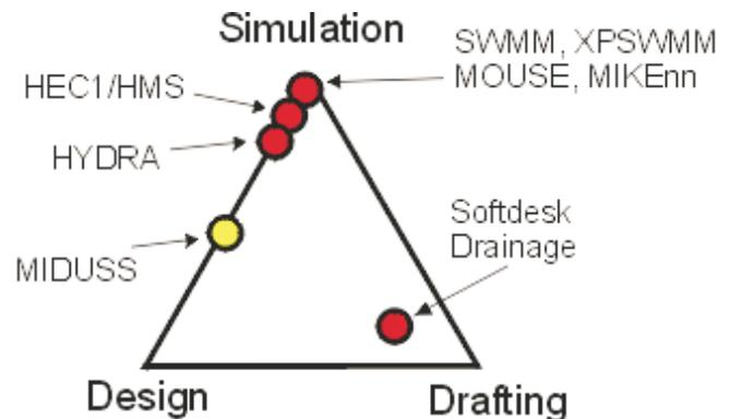
Interactive means that you design the network as the peak flow goes downstream. Each component can be optimized because you "interact" with the program so that the flow is conveyed in an efficient design. MIDUSS constantly provides you with feedback on how the design is going. If a pipe is surcharged, you will be told and encouraged to change the design.
